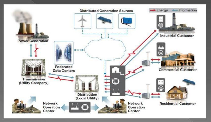
An intelligent electricity system that connects all supply grid (utilities) and demand elements (end-users) through an intelligent communication system
