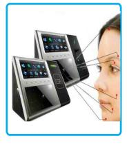
The technology used in F710 is called 'Dual Sensor' which combines the advantages of both 2D & 3D technologies. It uses two special cameras which are just like a person's eyes. The technology has fast recognition speed & high accuracy. Below given is the pictorial representation of 'Dual Sensor' technology.
