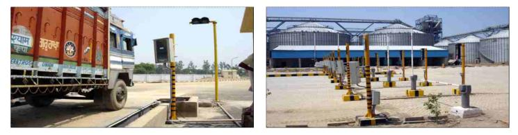
BGIL system identifies the vehicle authentication, lane demarcation and loading/unloading of the grains/goods as per the RFID tag issued to the driver after entering the requisite details in the BGIL software.
